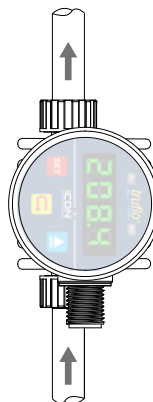
Vertical Mounted (Upward Flow)
